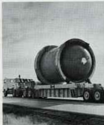
RIDING its Thiokol-built transporter, the forward segment moves to the Test Area for installation and assembly.
