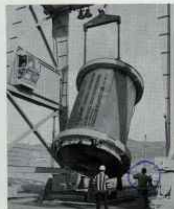
LOADED center segment is positioned on a special pallet by a 200-ton-capacity crane used to handle the giant loads.
